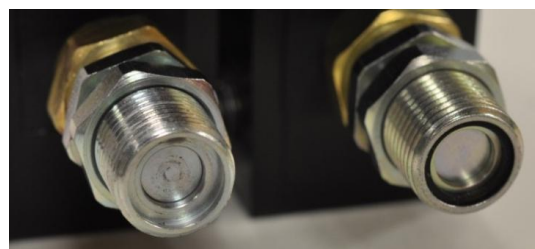
Left: Fitting missing O-ring
