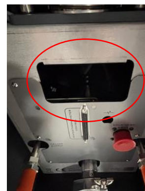
Step 5: After removing plastic wrap, use the handhold on the back panel (circled in red) to move the system
