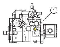
Figure 2-7. Drive Bypass Valve
