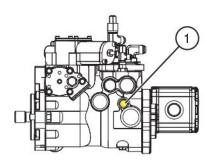
Figure 2-2. Drive Bypass Valve
