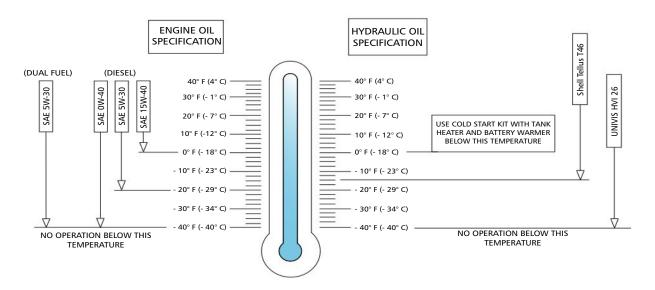
Figure 3-7. Cold Weather Operation Chart
