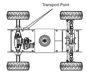
Figure 3-9. Turret Transportation Lock & Locking Points
