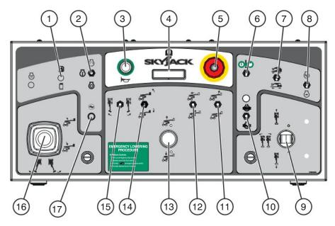
Figure 2-6. Platform Control Console
