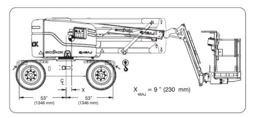
Figure 3-10. Lifting Points NOTE: Center of gravity varies with different options.
