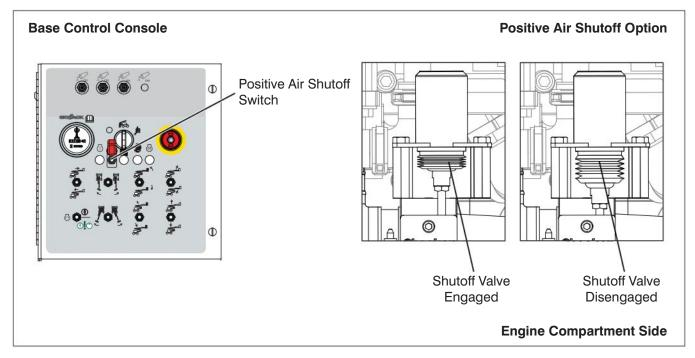
Test Positive Air Shutoff (If Equipped)
