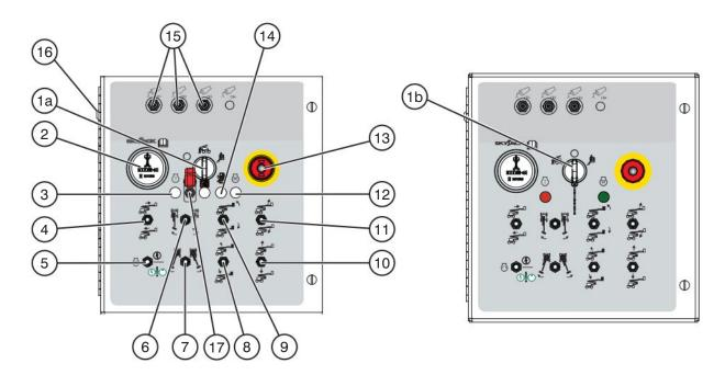
Figure 2-5. Base Control Console
