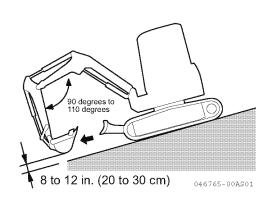
**2.** When climbing a slope, drive the machine with the implement positioned as shown in the right figure.
