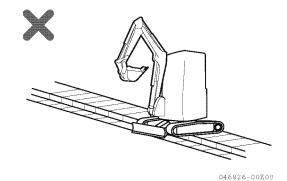
Do not steer the machine to a boundary between the flat ground and a slope while moving backward.
