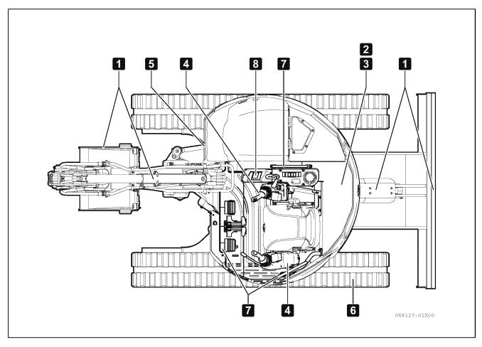
Check the implement, hydraulic cylinders, linkages, and hoses for damage, wear and loose connections. If any abnormality is found, take corrective action.
