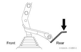
• When the blade is in the rear of the machine; Slowly push the travel levers 4 forward or step on the front of the pedals 5 to move the machine backward.
