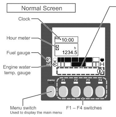
Function switch guidance Indicates the current functions of the F1 – F4 switches.
