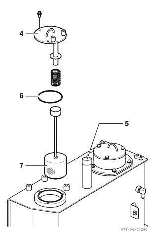
12. Put oil to the specified level through the oil supply port 5.
