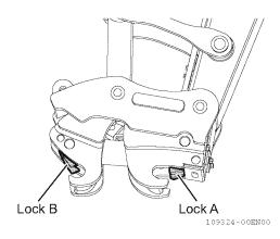
**1-** After mounting the attachment, check that lock A is in contact with the stopper and in the lock position.
