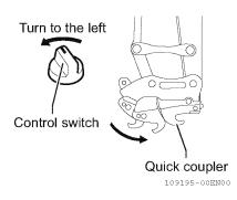
**6.** Remove the quick coupler from the attachment.
