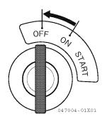
**4.** Set the starter switch to the "ON" position.
