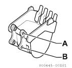
**5.** Clean the bucket boss section and install the O-ring.
