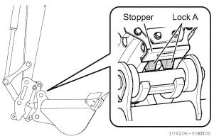
**2-**Set the implement in the position shown in the figure on the right and check that lock B is in contact with the stopper and in the lock position.
