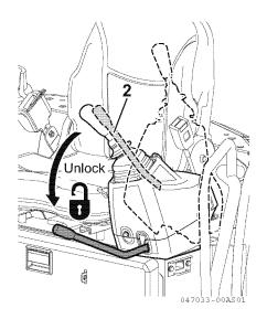
**4.** Set the lock lever **2** to the "LOCK" position to lock the control levers and pedals.
