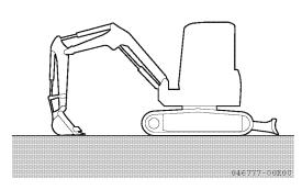
**5.** Set the lock lever **4** to the "LOCK" position.
