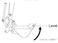
**6.** Turn the control switch right to the mounting position and mount the attachment.
