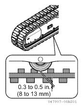
If the tension is improper, adjust it as follows:
