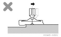
Steering the machine under this condition will cause the rubber track to come off.
