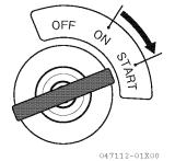
**4.** After the engine has started, release the starter switch key.
