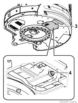
■ Checking the fuel level in the fuel tank and refueling
