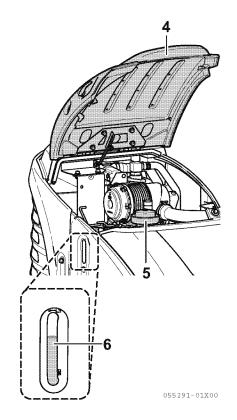
2. After refueling, securely retighten the fuel supply port cap, and close the engine hood B 4.
