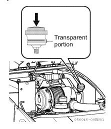
■ Checking and replenishing the engine oil
