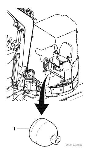
■ Releasing the internal pressure of the hydraulic circuit
