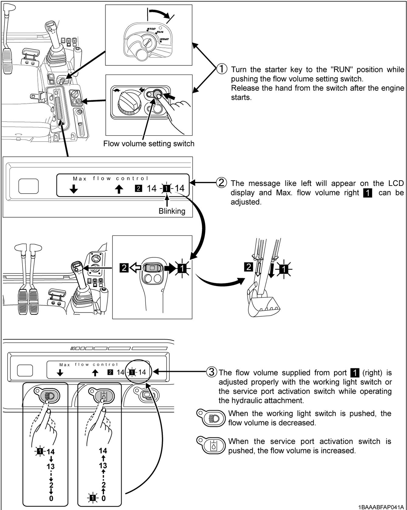
④ After Max. flow volume right **1** is set, push the display selector switch.
