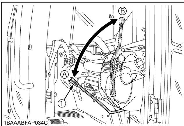
(1) Lock lever for control lever (A) "Unlock"
