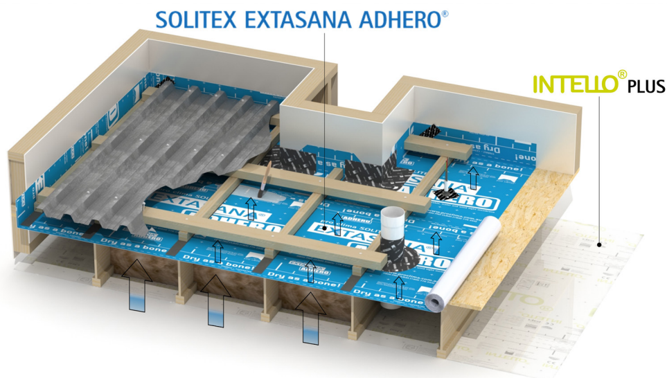
Figure 11, Typical ventilated low-pitch roof construction (Recommended)
