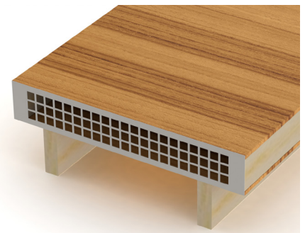
Figure 2 – Opening B (69% open)
