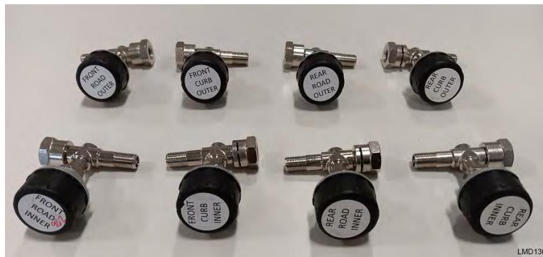
Figure 16 TPMS Sensor labeled
