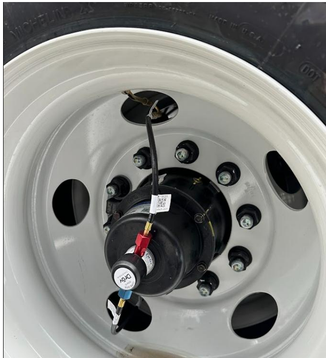
Figure 43 Installed rotary union with hoses
