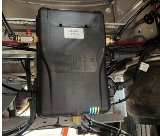
Figure 5 AirBoxOne Mounting example
