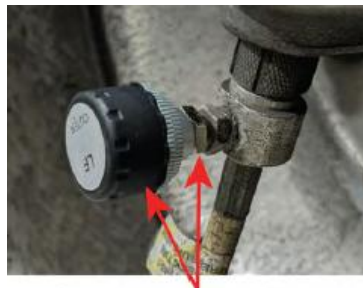
Sensor and Jam Nut on Junction
