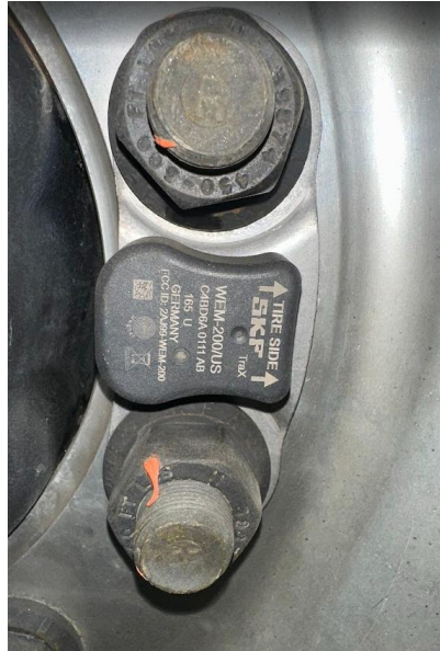
Figure 51 SKF Sensor Installation Example
