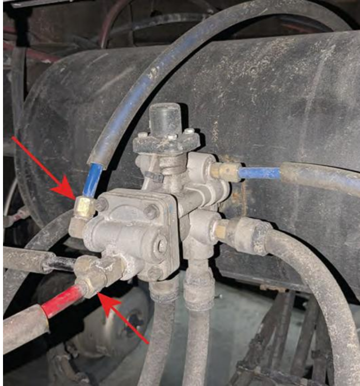
Figure 18 Brake Pressure Sensor location
