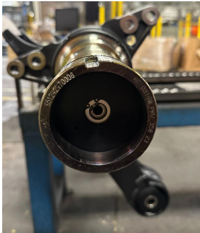
Figure 41 Axle Plug install
