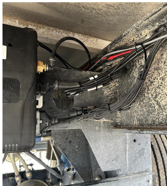
Figure 32 Wire routing example
