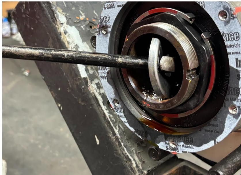
Figure 38 Lever using pry bar
