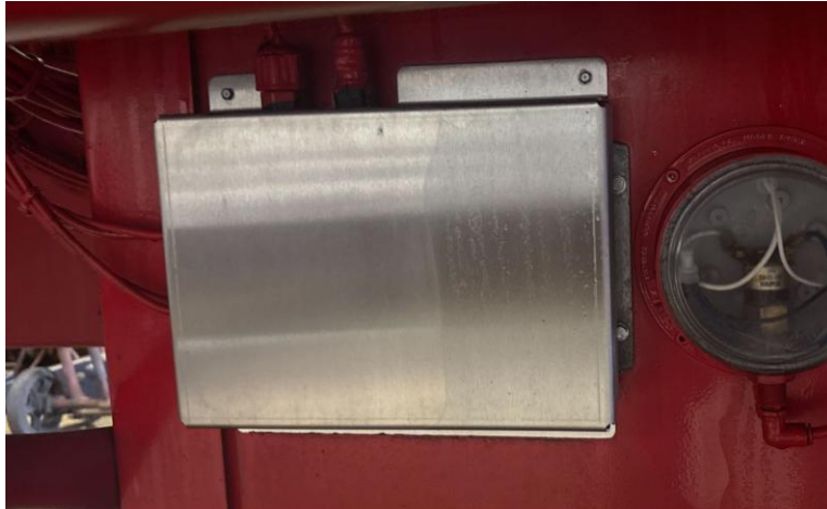
Figure 12 Cover placement over VCU
