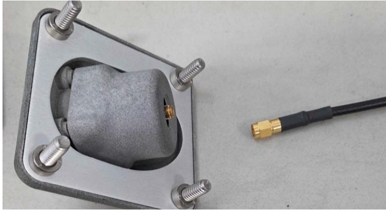
Figure 40 Cable fully separated from the camera after sleeve removal
