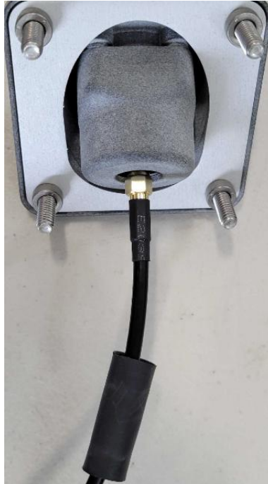
Figure 35 Cable connected to the camera and torqued to 8 in-lb.
