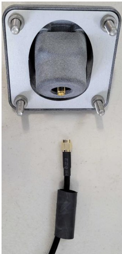
Figure 34 Heat shrink staged on cable before mating to the camera.
