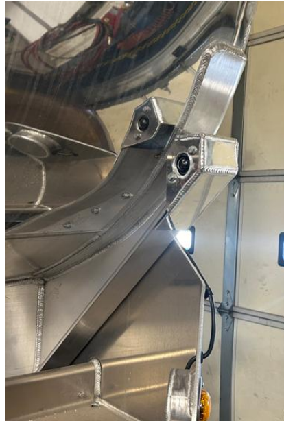
Figure 3 Sensor Unit Mounting example
