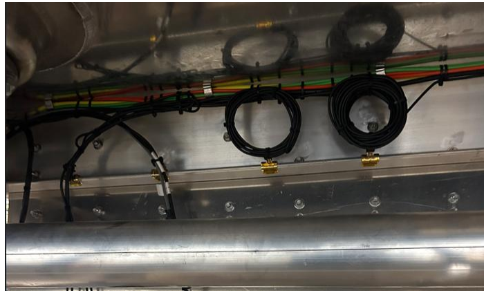
Figure 15 Wire Routing Example
