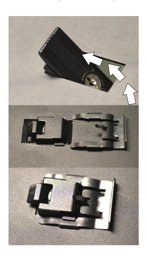
The key latch body is installed from the back of the door and secured by pushing the spring clip under the protruding ears and snapping the back edge into the latch cutout in the door. Two keys are included with each latch and all latches are keyed alike.
