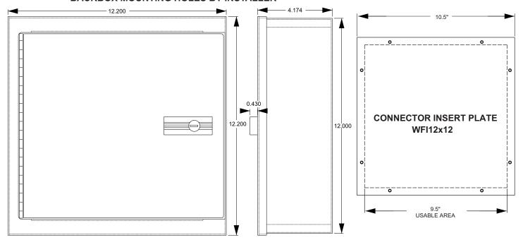
Both the door and the connector plate attach to the separate black recess frame. The door attaches to the top and bottom of the frame, which must be mounted to the 12X12" back box so that the holes for the cover mounting screws are positioned correctly. Mounting holes for the frame are provided on all four edges and it is recommended that screws be installed in each side. Flathead screws (SCR832X3/8FPU) are included.
