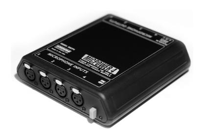
The Whirlwind Micpower 4 (MICP4) is a premium four channel phantom power supply. The regulated 48 Volt DC output is ultra quiet, introducing no noise into the microphones' signal path. The Micpower 4 uses an external AC adapter (PS24AC) to eliminate magnetic fields generated when using an internal transformer type supply. The sleek, rugged design is perfect for any application when the use of high quality microphones require the use of external phantom power.
