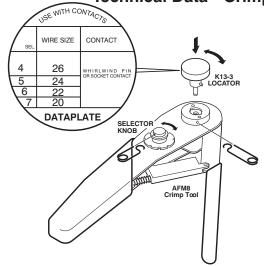
The W3RP is a rear insert, rear release crimp type connector. Contacts are loaded into the insert body and removed from the rear (wiring side) of the housing. To prepare the wires for use, follow the diagram for removing the jacket and the foil shield from the cable pair. Be careful not to nick and do not tin the ends of the wire being stripped. Insulate the drain wires with the clear PVC tubing and use the heat shrink tubing over the foil of each pair.
