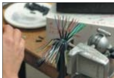
The right way to prep a MASS connector, keeping things organized and secure.
