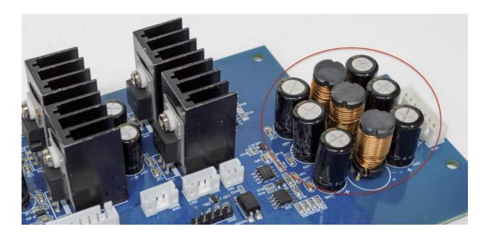
A CLC filter is a passive circuit using two capacitors and an inductor to reduce noise and ripple in power supplies and signal paths. It works by shunting high-frequency noise to ground (C1), blocking AC components while allowing DC to pass (L), and further smoothing the output (C2). This design provides superior ripple reduction, better efficiency than RC filters, and stable power delivery, making it ideal for high-performance audio amplifiers, DACs, and power supplies.
