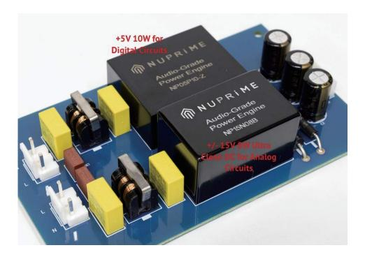
The NuPrime custom-designed DC converters, NP15N08B and NP05P10-Z, provide separate, optimized power supplies for analog and digital circuits, offering distinct benefits. The NP15N08B delivers +/- 15V at 8W for analog circuits, while the NP05P10-Z provides +5V at 10W for digital circuits. By isolating these power supplies, digital noise and interference are prevented from contaminating the analog signal, helping to preserve the purity and fidelity of the audio output.
