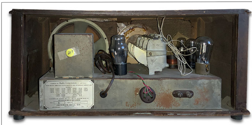
Model 6 rear view showing the speaker plug and chassis mounted speaker, licensing plate, and the ground and antenna connectors.
