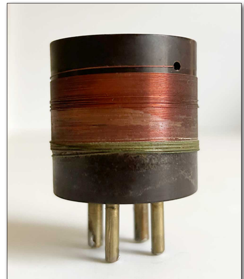
Type of coil installed on the Model 8 (2 on the top, 2 under the chassis)
