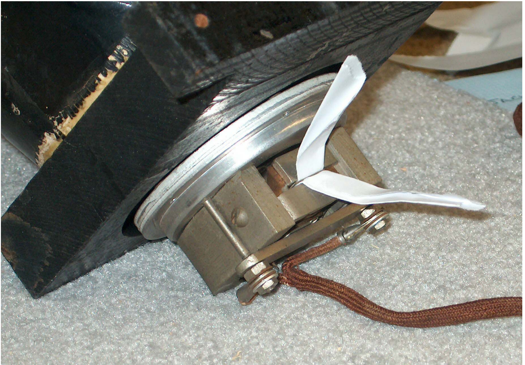
The Armature was pressed against the pole piece. A paper slim was used to center the armature, and the bolts re-tightened
