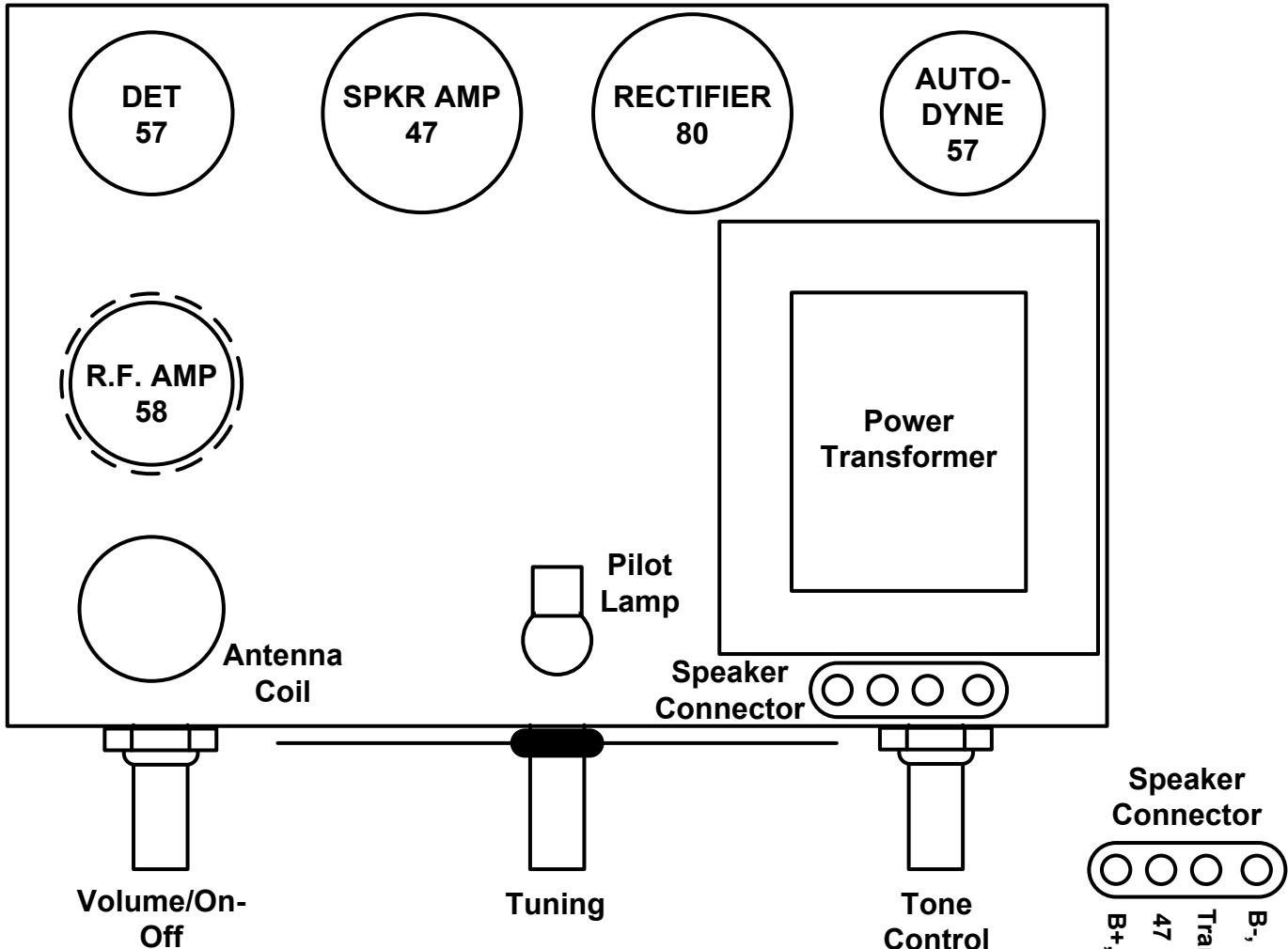
The Tuning Condenser is mounted below the Chassis
