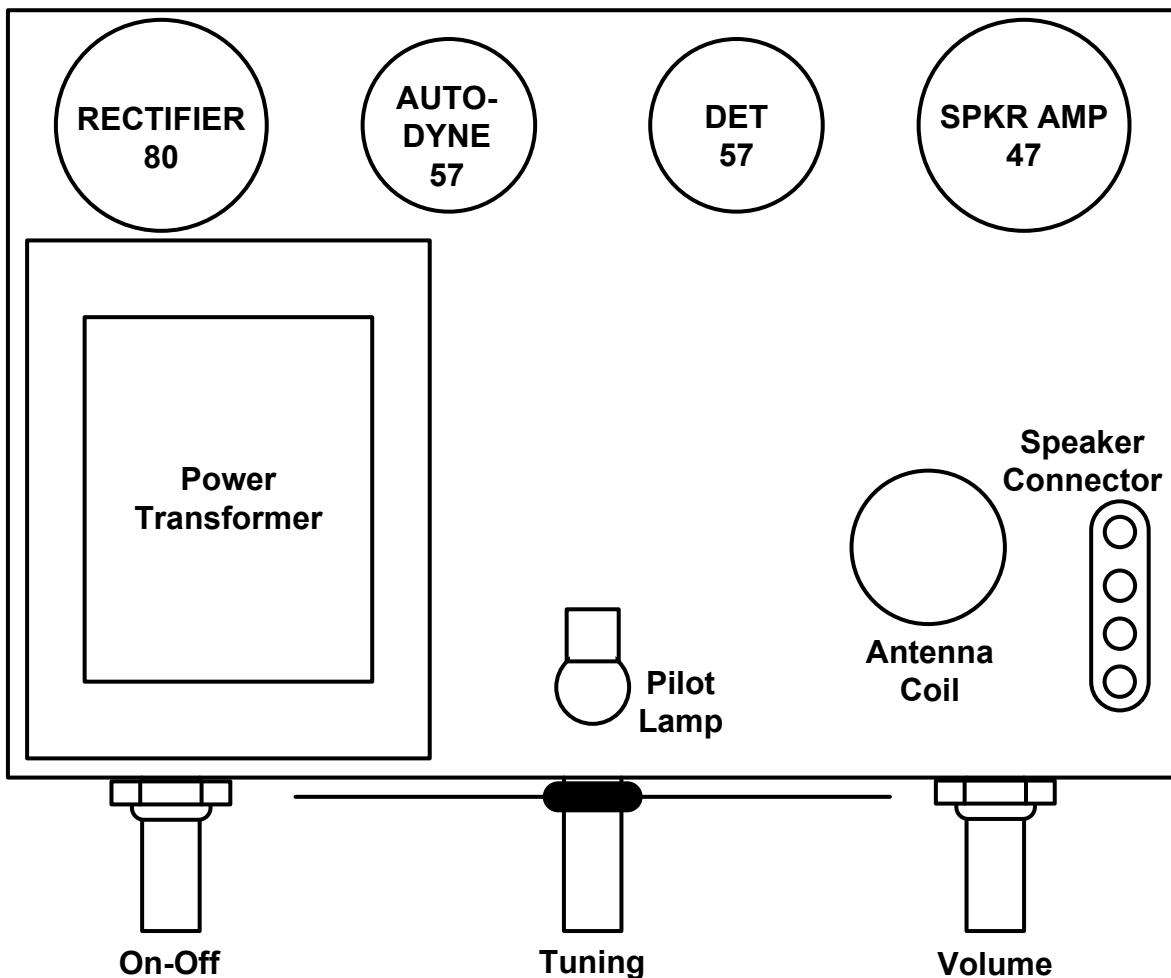
The Tuning Condenser is mounted below the Chassis
