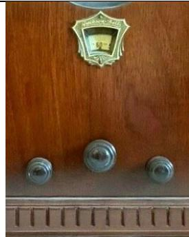
**Outer Rim Drive** with an Escutcheon was used on the first Jackson-Bell Superheterodyne
