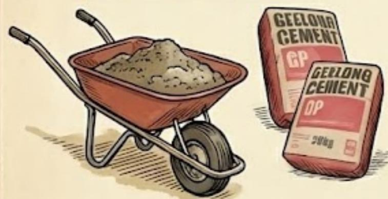
MIXTURE: SOIL FROM HOLE + 2 SHOVELS OF CEMENT (1/4 BAG) + 8-12 LITRES WATER. AIM FOR THICK CREAM CONSISTENCY.
