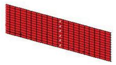
Mark a line on fold on Speedform with a pen. Leave the top wire intact and cut alternate wires (x) for width of unit.
