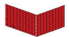
Fold the Speedform on a bench or on the ground. A suitable timber straight edge may be used to assist with the folding. Cutting every other wire at the fold point makes Speedform easy to bend on site.
