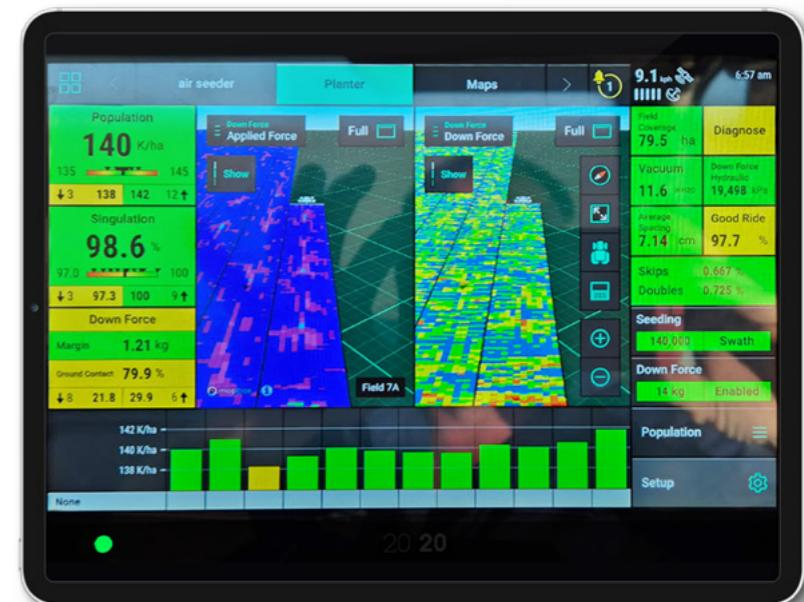
for depth and spacing, with accurate downforce applied to ensure uniform planting depth, seeking to achieve up to 98% accuracy. The system measures seeding rates and, if necessary, issues an alert to the driver to take corrective action. This technology enables precise planting and high uniformity, which helps maximise yields and lowers production costs.
