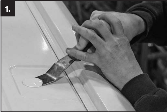
1. Carefully remove rubber plugs for the openings.
