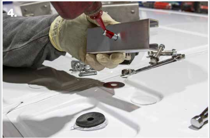
4. Place rubber fender washer over bead of caulk around each opening. Put a few drops of red Lok-Tite thread locker on the 8 mm bolt threads.
