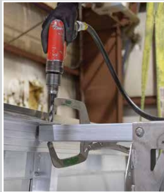
Drill 3/8" Hole Between Angle and Crossbar
