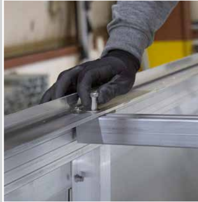
Insert Bolts through Mounting Angle and Roof Rack Crossbar
