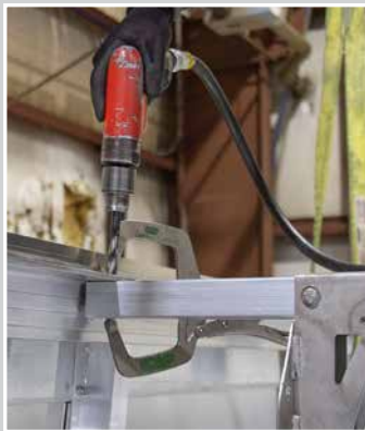
Drill 3/8" Hole Between Angle and Crossbar
