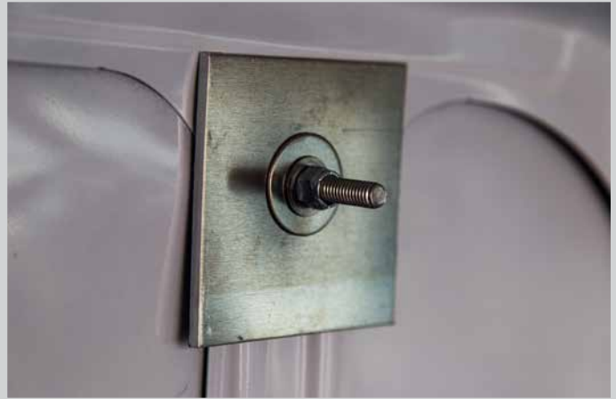
4" x 4" reinforcement plate between sprinters interior wall and washer and nut.
