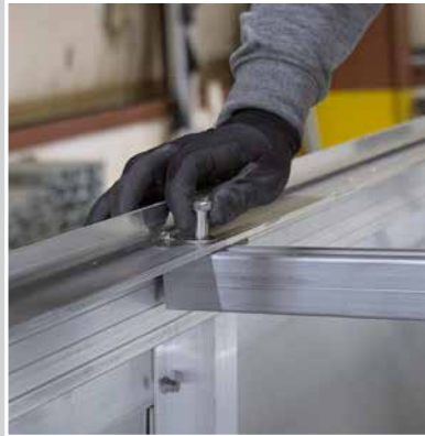
Insert Bolts through Mounting Angle and Roof Rack Crossbar
