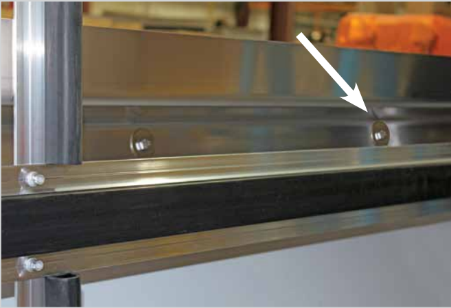
Bolt through mounting channel attached to glass rack.
