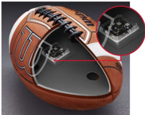
UWB microchips track precise location data
