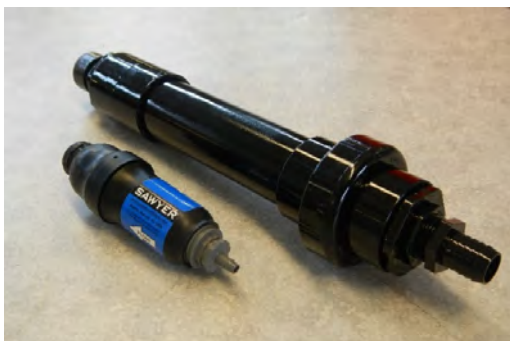
Figure 42: Prototype 2.0 – Size Comparison with Sawyer® Filter and Custom-made Acrylic Joint
