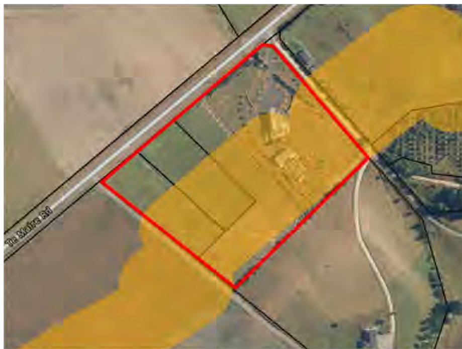
Figure 1: Fault Hazard Area (orange area) on 139, 155 and 157 Te Maire Road (red outline)
