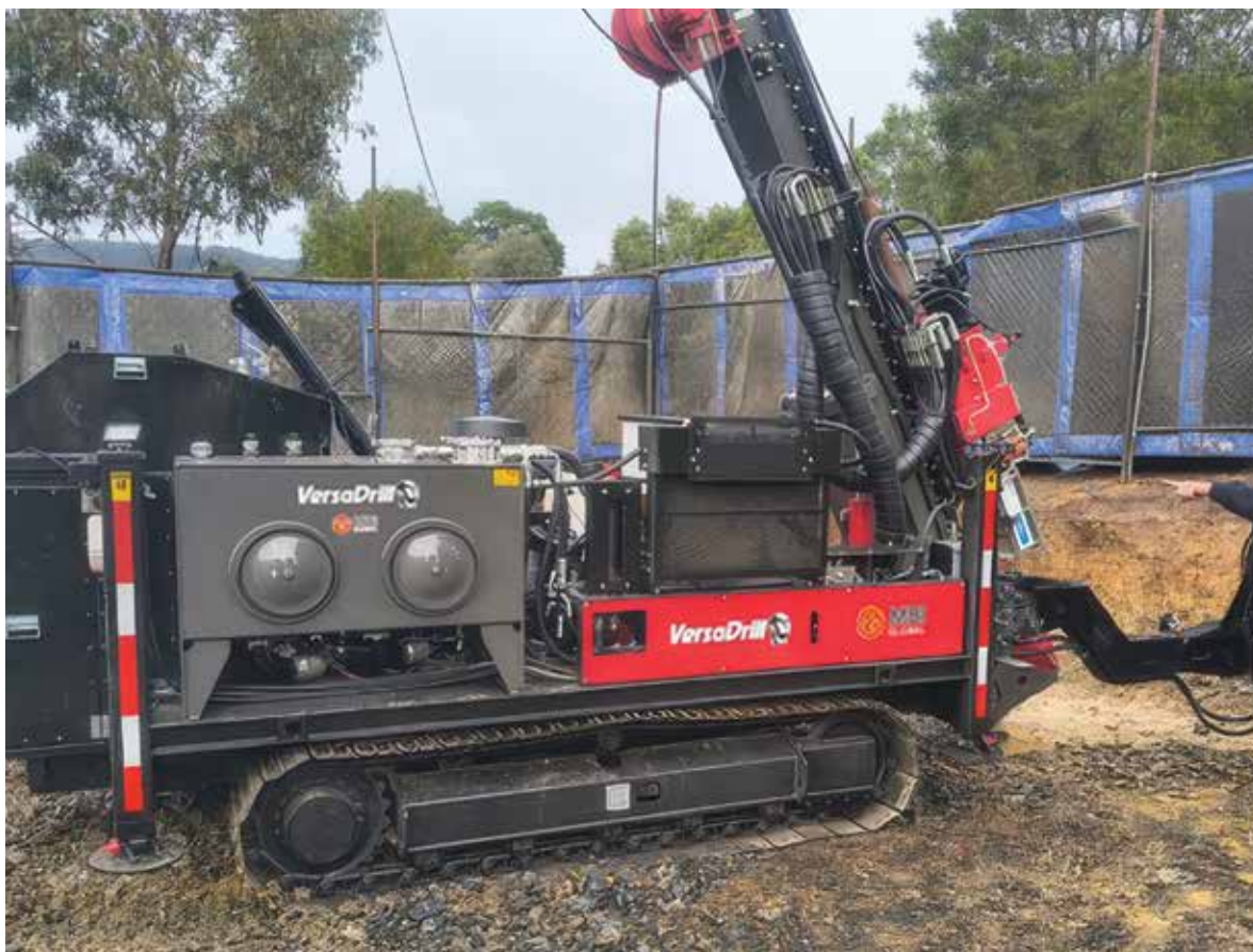
MBI Global and Star West Drilling developed this low-footprint drill rig specifically for Sunday Creek. Southern Cross Gold says the Australian-first asset reduces drill-pad footprint and noise while retaining the capacity for deeper, precision drilling. Photo: Southern Cross Gold Consolidated.
