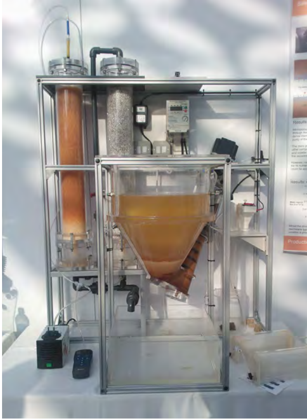
Solid-liquid separation and diffusion of water through hydrophobic membranes in the front unit. © SuSanA Secretariat_ Flickr_CC
