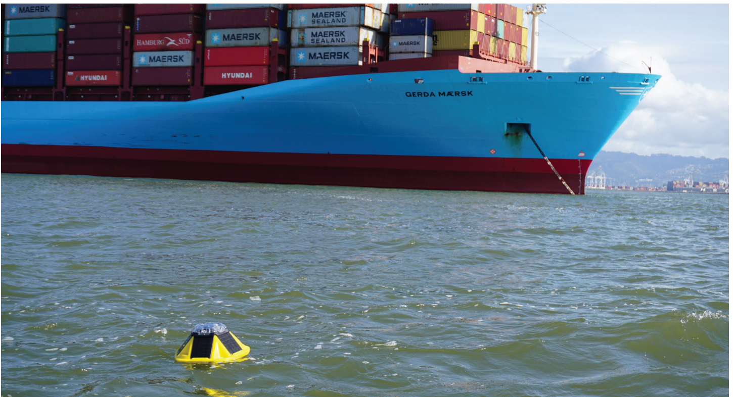
Sofar's Spotter buoys collect and transmit wave, wind, sea surface temperature, and barometric pressure data.
