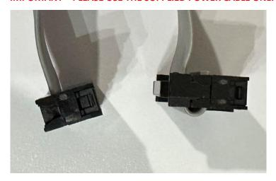
The cable on the left is the supplied power cable that doesn't have a strain relief attached.
