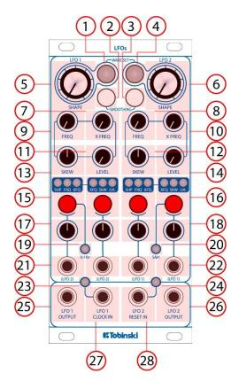
1 and 4, WAVE SET – LED Switches to select the wave set bank and display the LFO tempo. The LED colour indicates the selected wave set (yellow for bank A and red for bank B).
