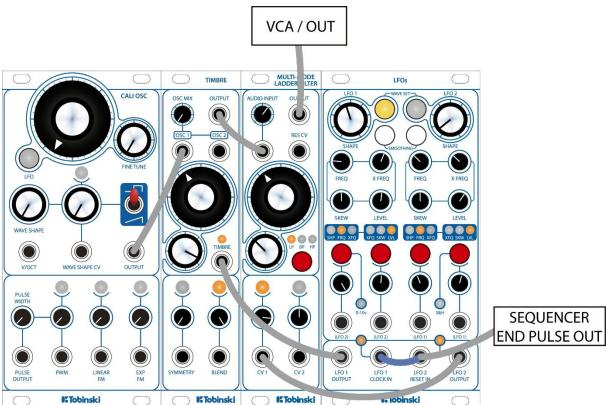
This patch is used to demonstrate some chaotic type modulation using the cross-modulation of the LFOs and a reset pulse from a sequencer or drum machine etc so that the modulation can achieve some kind of rhythmic pattern. Setting the reset pulse to 1 or more bars is best as it gives the LFOs time to form a rhythmic pattern before being reset.
