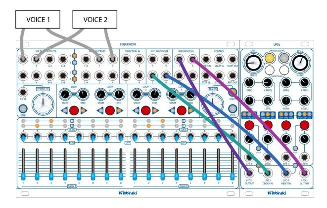
The purpose of this patch is to generate some interesting unquantized rhythmic variations that are synced to the first beat of the bar but are not locked the standard timing grid within the bar.
