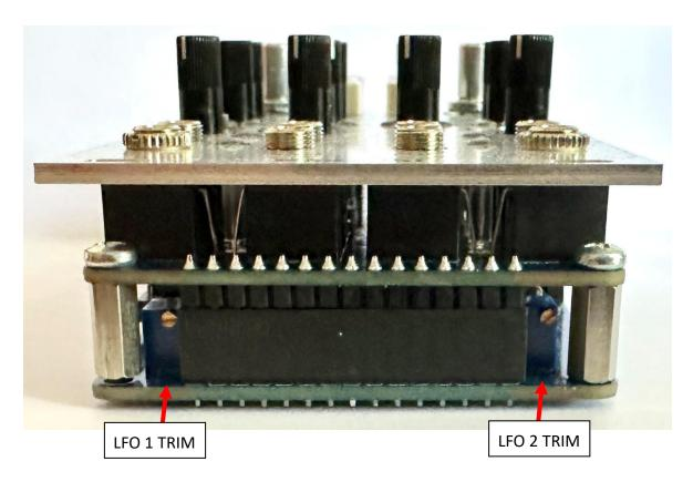
The calibration for each LFO removes the dc offset so that the LFOs are centred around 0V. The procedure is exactly the same for each LFO.
