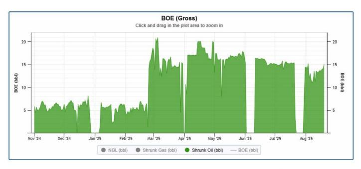
03-02 well with significantly increased production after waterflood pattern change and well speed-up to 3x RPM.
