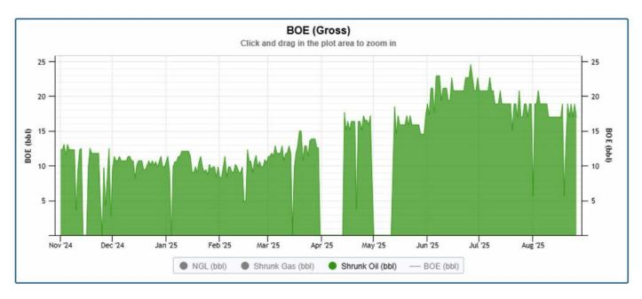
03-30 well, optimized through reduced water injection into nearby wells and slowing down RPM of well thus significantly increasing netbacks.
