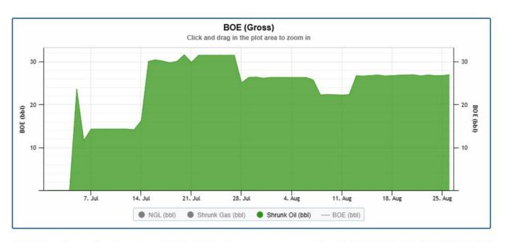
10-07 well producing steadily for 50+ days now, currently at 90 RPM with 10 JOF (Joints of Fluid) optimization potential. Casing pressure continues to climb, now at 30 PSI showing strong reservoir drive.
