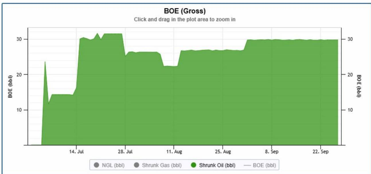
*10-07 well producing steadily for 75+ days now, currently at 100 RPM with 12 JOF (Joints of Fluid) optimization potential. Casing pressure holding steady at 30 PSI.*
