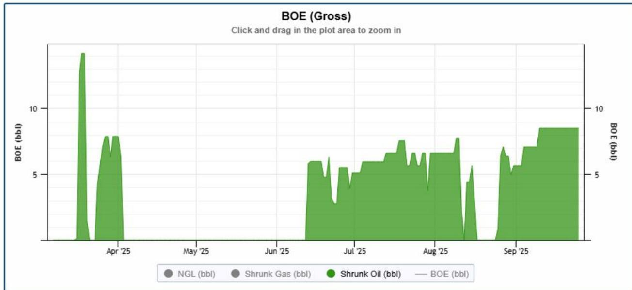
*02-33 well, one of our focus wells in Section 33 which is currently at 3% Recovery Factor. Previous attempts to run this well have caused major sand influx, so an enhanced recycle pump and sand suspension chemical setup were installed.*
