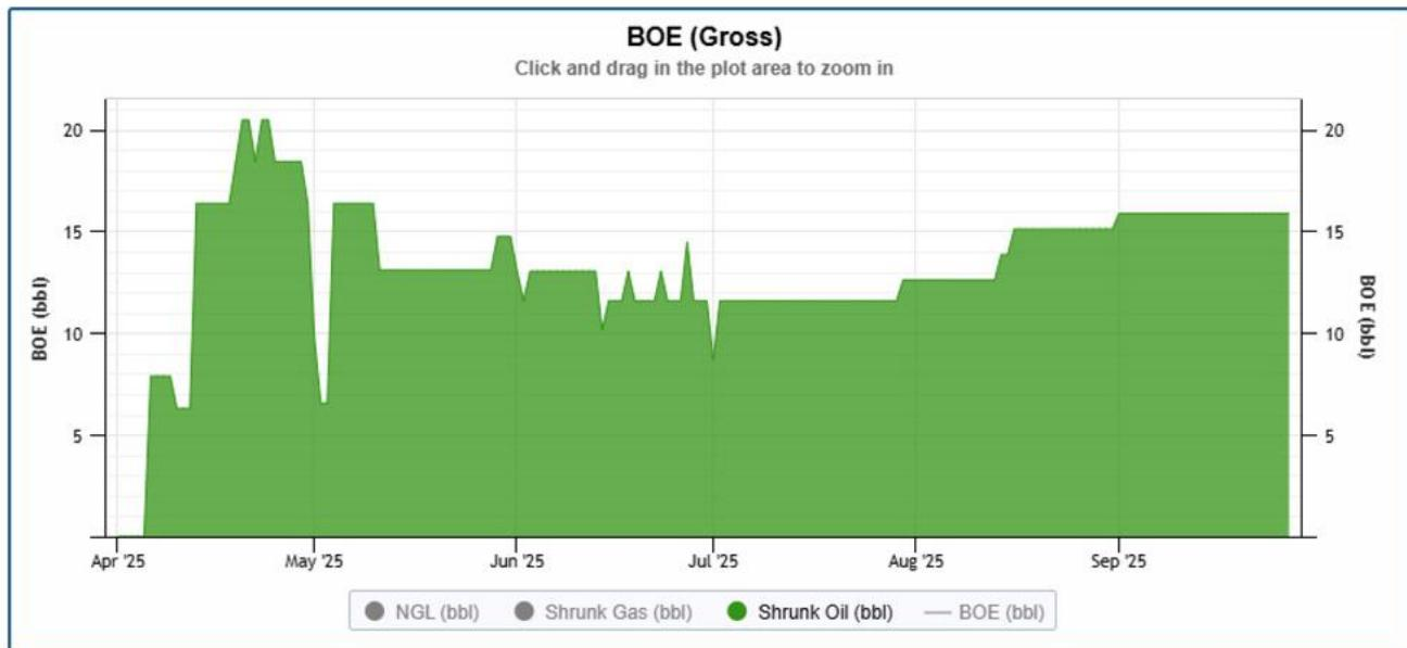
*01-17 well with constant production profile in the last 6 months through small speed-ups. This well sits against the updip erosional edge of Luseland pool and produces at a very low water cut generating exceptional netbacks.*
