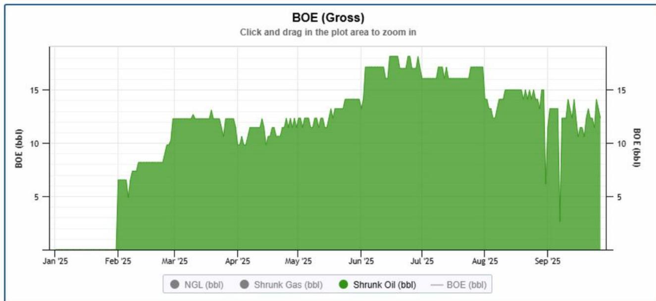
*04-34 well reactivated after 4 years offline. Optimizing through speed-ups as production stabilizes and accessing bank oil at reservoir edge.*
