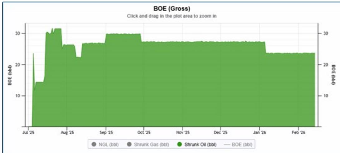
10-07 continues to be our star well and a model of consistency. After more than seven months of steady output with stable oil cuts, it still holds significant optimization potential. We are confident that with further adjustments, we can unlock even more value from this reliable producer while carefully balancing total fluid production to prevent water coning.
