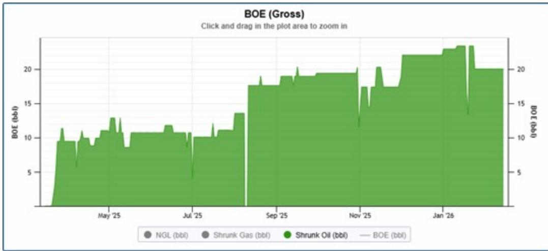
10-08 is a strong testament to the effectiveness of our optimization strategy. Through careful operational management and incremental RPM increases, we have successfully increased oil production while reducing water cut. We will continue to closely monitor performance to maximize output as oil cuts improve and oil viscosity decreases through ongoing incremental wormhole propagation.
