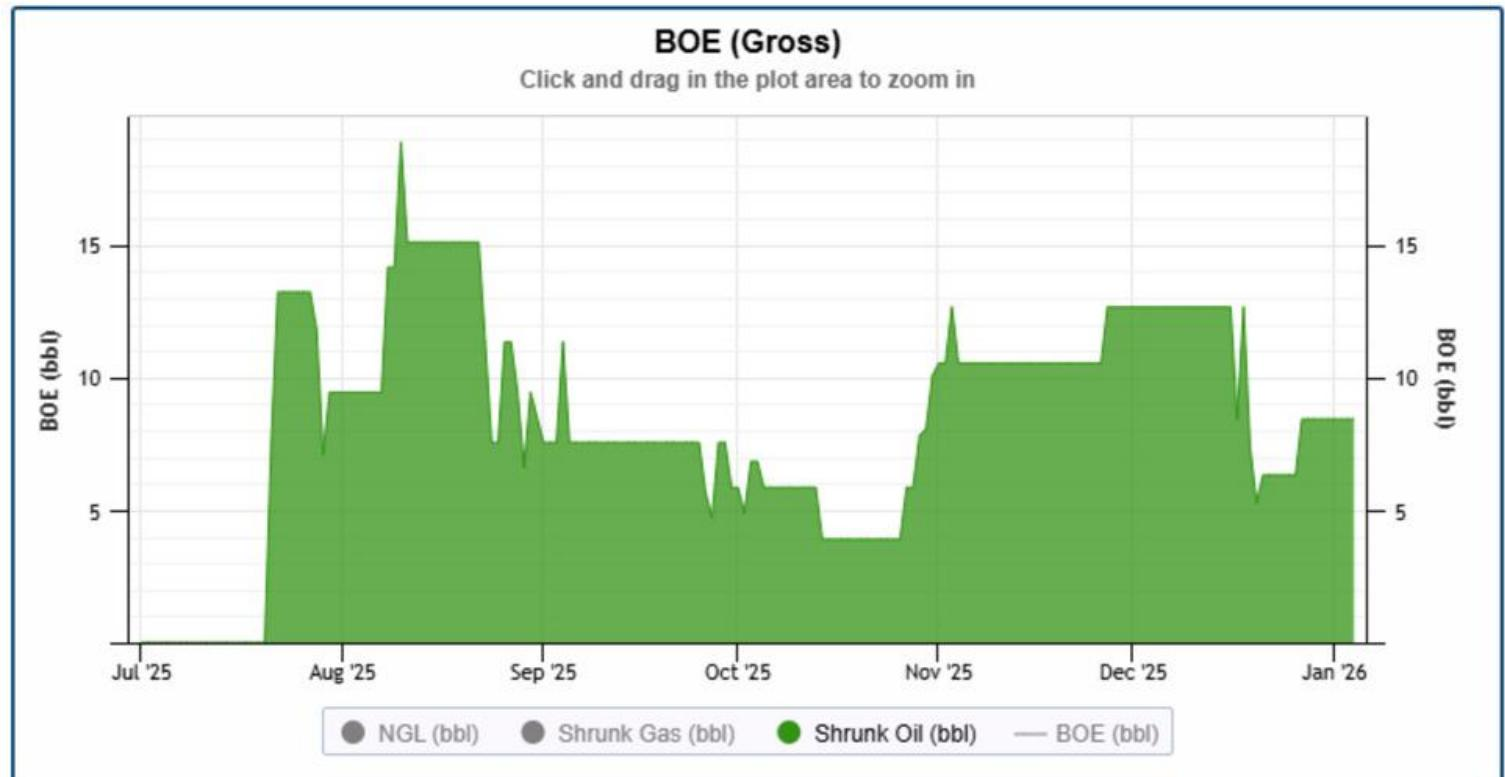
12-17 well, one of our most recent reactivations, is now approximately 180 days online and exhibiting sand-slugging behavior. A recycle pump has been installed and is currently operating under a program of steadily increasing daily hot oil injection, alongside incremental well speed-ups. The team is carefully optimizing operations as well and fluid levels continue to fluctuate on a day-to-day basis.
