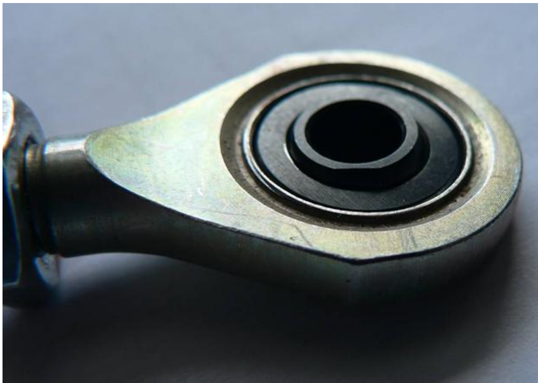
Fig. 2 Unsatisfactory method of securing the bearing in the eye
