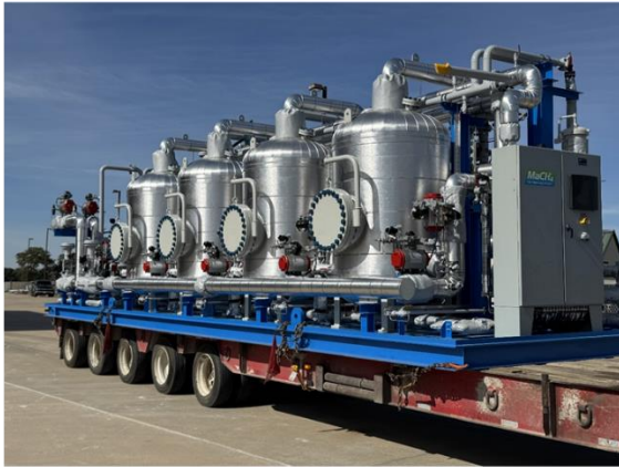
Fig. 9 – The commercial system has an inlet capacity of 2,500 Mscfd and fuel gas capacity of 1,500 Mscfd while being able to be easily moved to a compressor station.
