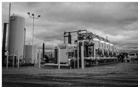
Fig. 11 – The commercial system demonstrated the ability to deliver less than 1,070 BTU fuel gas at the initial installation site in Beckham County, Oklahoma
