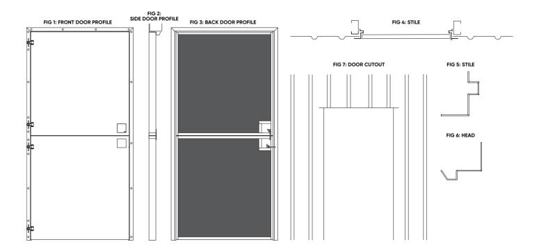
The Sentry<sup>™</sup> 801.47 stable door is a metal-clad door, comprising of RHS frame with a steel skin and internal 18mm black ply cladding, pre-hung into a 47 series 3-sided jamb.
