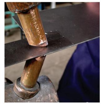
Hold the work pieces securely against the lower electrode.
