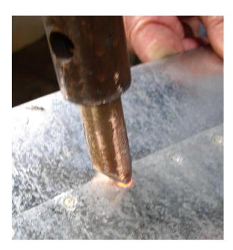
Close the upper electrode down firmly to initiate the welding current circuit and join the work pieces.
