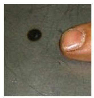
Allow the joint-spot to cool. Check each spot weld is firmly joined and measures approximately 6 mm – 8 mm.
