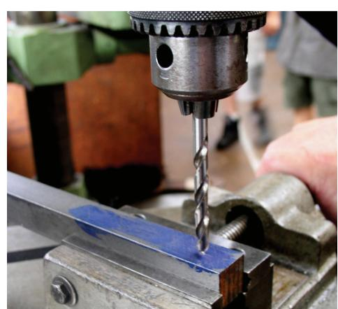
When ready, pull down steadily and lightly on the feed handle.
