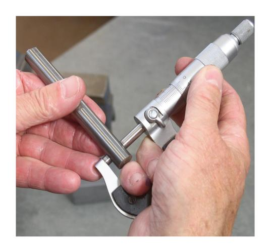
Using a micrometer or vernier calipers, select the correct size bar for the thread to be cut e.g;
