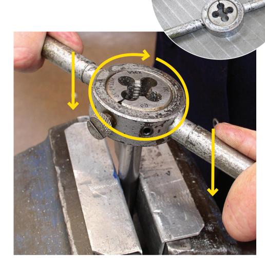
Typically it takes **two** cuts to form an external thread, a rough followed by a finishing cut. To start the first cut, hold the bar vertical in a vice with the chamfered end up.
