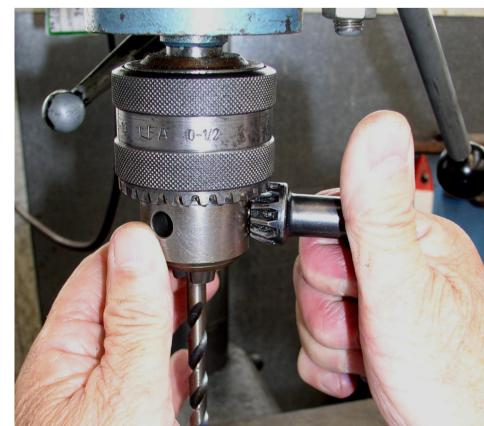
Ensure there is at least 25 mm of shank in the chuck and it is firmly tightened.
