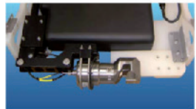
CABLE CUTTER SKID
