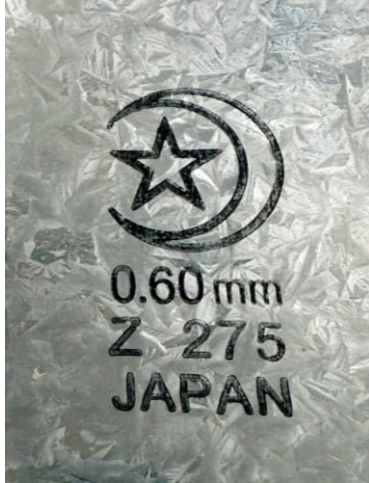
Figure 1 Sample Product Surface Marking (0.60mm / Z 275) Showing brand marking, thickness and coating information
