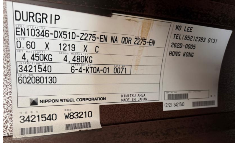
Figure 2 Sample Product Label (0.60 x 1219 x C) Showing product specification, dimensions, weight and traceability information
