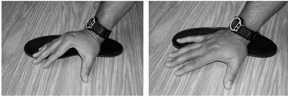
Fig 1. Hand configurations (postures) used for manipulation trials demonstrating the pressure sensor pad: arched configuration (left) and flat configuration (right).
