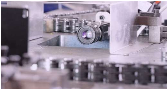
All chains are produced on an automated assembly and online inspection line with pre-stretching, boosting fatigue strength while ensuring perfect straightness for flawless assembly.
