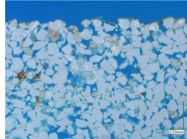
Figure : Sample after 5 day breaker soak
