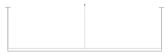
Dims: 2500 mm L, 45mm H, 35mm D Weight: 2.2kg
