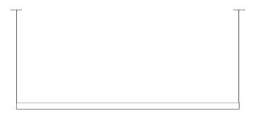
Dims: 1600 mm L, 45mm H, 35mm D Weight: 1.6kg
