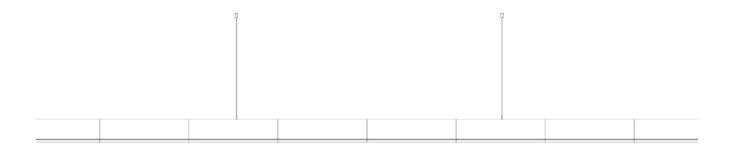
Dims: 2410 mm L, 58mm H, 58mm D Weight: 16kg
