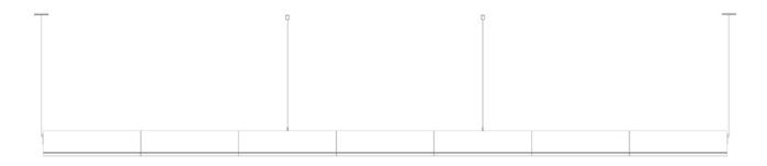
Dims: 2110 mm L, 58mm H, 58mm D Weight: 14kg
