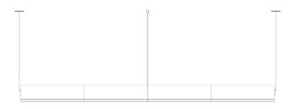
Dims: 1210 mm L, 58mm H, 58mm D Weight: 8kg
