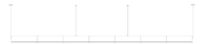
Dims: 2110 mm L, 76mm H, 62mm D Weight: 14kg
