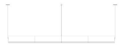
Dims: 1210 mm L, 76mm H, 62mm D Weight: 8kg
