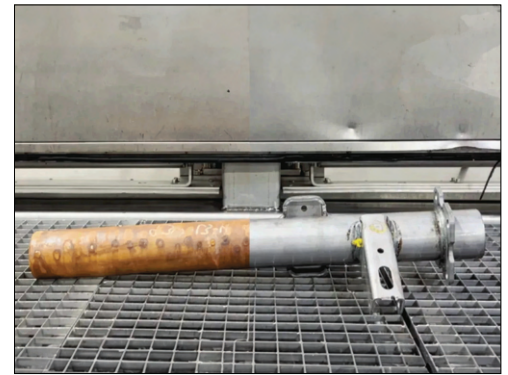
Value 3 – Photo of partially derusted axle tube for process reference.
