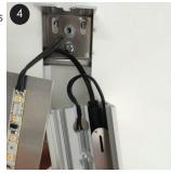
5. Slide Jut onto bracket & secure with set screw on top.
