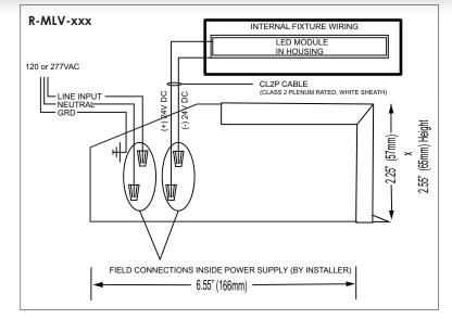
1. Mount housing on studs, blocking or into cutout in existing wall & run CL2P wire to remote power supply.
