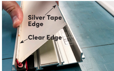
Step 6: At an angle, push the CLEAR (Fig. A) side of Acrylic Light Guide against the LEDs & center the length. Then rotate & push flat into position.
